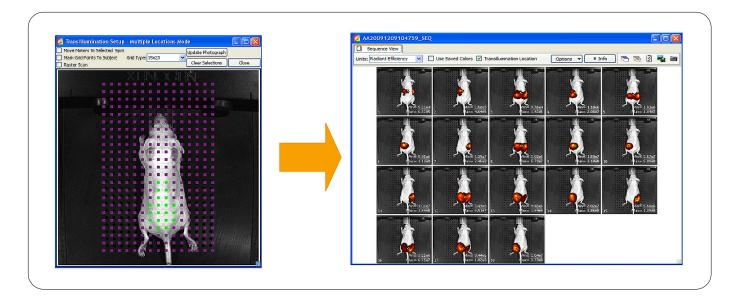
With transillumination raster scans, the shutter remains open as the source moves from point to point. This results in one image as seen below and saves the user time. Whole mouse imaging times are now in the range of 2-5 minutes depending on the intensity of your probe.
