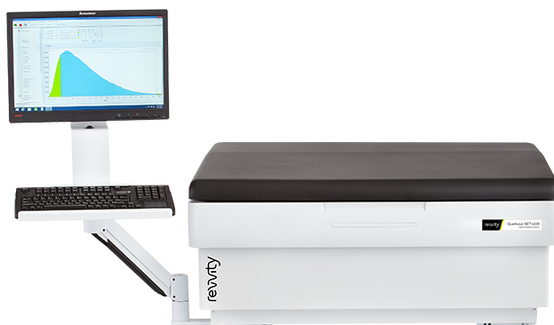
Instrument - A Quantulus GCT 6220 equipped with QuantaSmart 5.2 software, including PSA based alpha/beta separation and histogram electronics.
