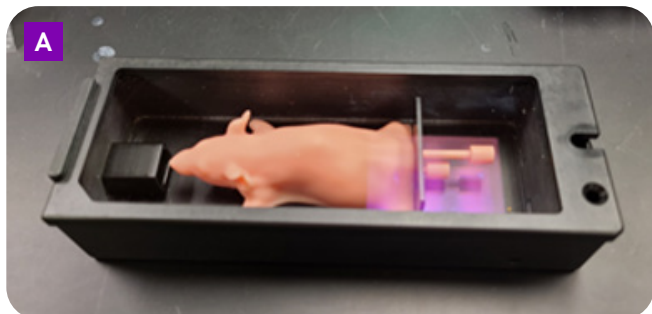
Figure 2A: The mouse imaging shuttle (MIS) allows an anesthetized mouse to be transferred from the IVIS Spectrum 2 to the Quantum GX3, enabling co-registration of optical and advanced microCT images.
