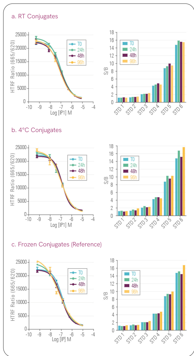
Figure 2: Stability of working solutions of detection reagents (IP1-d2 and Ab-K conjugates) is shown by comparing HTRF ratios and S/B over time after storage at a. RT, b. 4°C and c. frozen (reference). Small signal modulations after room temperature and 4°C storage are not significant (also seen in frozen reference). Note: S/B STDx = HTRF Ratio STD0 (= Max Signal) / HTRF Ratio STDx
