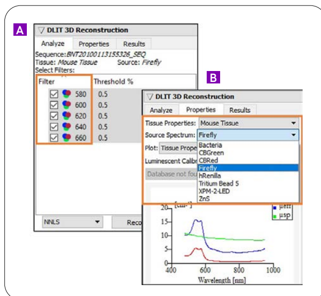
Figure 2: A) Living Image automatically selects the filtered images that have good quality for reconstruction. B) The Properties tab allows you to choose the tissue properties and bioluminescent source.
