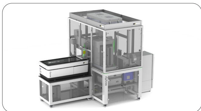
Figure 5: Example for an explorer™ G3 workstation for an integrated and fully automated workflow for a complete hands-free and standardized high-content toxicity assay with GrowDex-embedded HepG2 spheroids described in here. This automation solution includes for example a JANUS G3 automated liquid handler, cell culture incubator, centrifuge, sealer/peeler, Opera Phenix Plus and Celigo® image cytometer.
