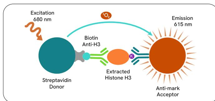
Figure 1: Schematic representation of the AlphaLISA cellular assay for the detection of modified histone proteins.
