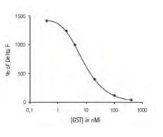
The GST check kit enables the verification of tag accessibility on GST-tagged fusion proteins. The graph alongside shows the dose response curves of different GST fusion proteins.
