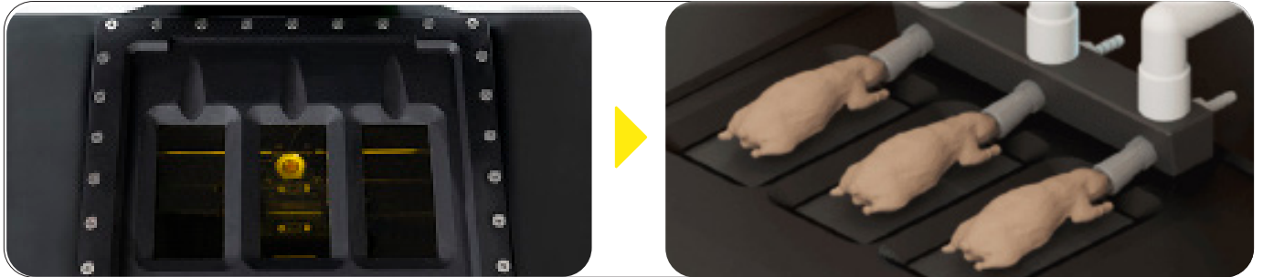
Figure 6: (Top) Imaging stage showing 3 mouse imaging bay. (Bottom) Imaging stage displaying mice in each bay.
