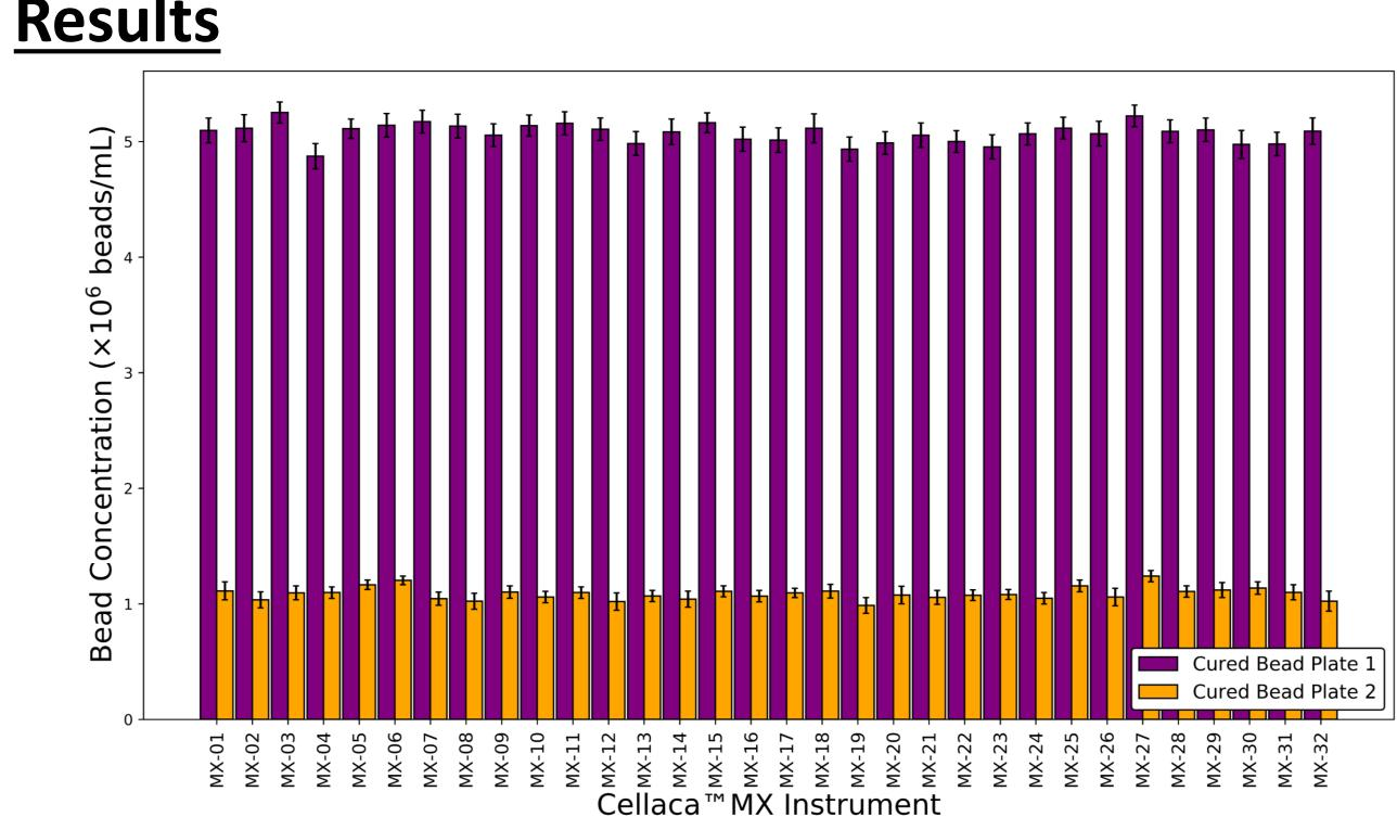
The CV of the method as whole (~3000 counts, 96 wells, 4 plates, 32 instruments) was 5.7%.
