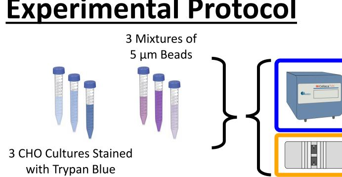
We measured 3 CHO samples and 3 bead samples using the Cellaca<sup>™</sup> MX and a hemocytometer.
