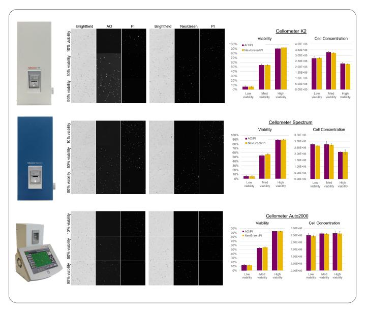
Cellometer™ K2, Auto2000™, and Spectrum™ systems results are similar and show that viabilities of Jurkat cells match within 5% of each other independent of sample type (low, intermediate, or high viability), while cell concentrations differ up to 6% when comparing NexGreen/PI and AO/PI.
