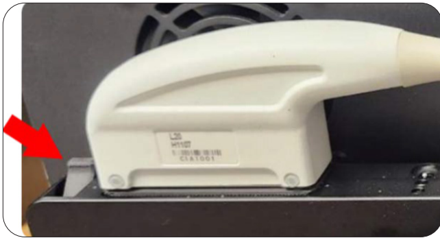
Figure 2: Transducer cable and connector. The connector lock is highlighted with a red arrow. Note the orientation of the transducer relative to the connector lock.
