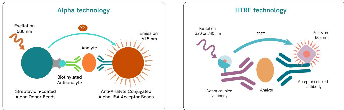
**Alpha** is a versatile, bead-based platform that enables you to assay the most complex samples in one well and with no wash steps.
