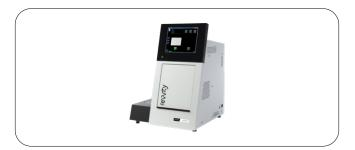
LabChip® GXII Touch™ - Microfluidic capillary electrophoresis on the LabChip GXII Touch, combined with consumables and reagents provides rapid, reliable and quantitative protein and nucleic acid analysis for a variety of virus related applications: QC of mRNA/DNA/protein vaccines, characterization of antibody therapeutics in between analysis of virus-like particles.
