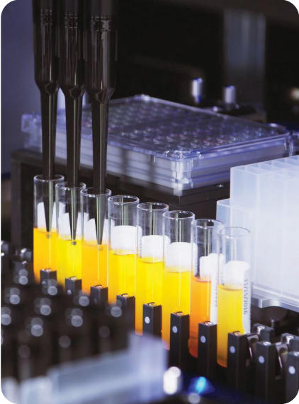
Automated plasma pipetting helps avoid contamination.
