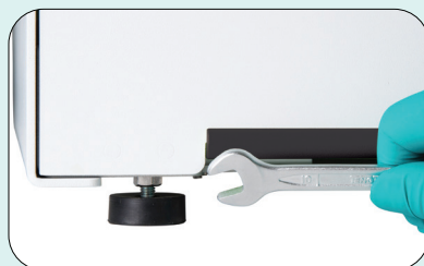
| Level the instrument with leveling tools
