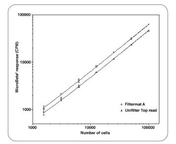
Figure 3. **<sup>3</sup>H-Thymidine labeled Jurkat cells harvested on a glass fiber filter** and measured with the MicroBeta<sup>2</sup> Microplate Counter. Both Filtermat A and Unifilter plate had a very good linear correlation (R=0.9999) over a wide range of cell numbers.
