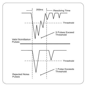
Figure 1. In High sensitivity TR-LSC mode, at least three individual pulses must cross the threshold to register a count. This prevents any randomly occurring single background pulses produced by thermal noise to trigger a count.
