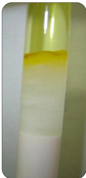
Figure 2: Glass column filled with aluminum oxide at the bottom and Silica on top of the column
