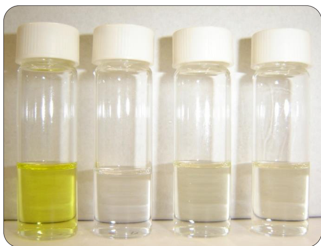
Figure 3: Decolorized samples of biodiesel dissolved in heptane
