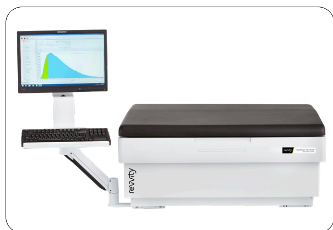
Figure 1: Quantulus GCT 6220 liquid scintillation counter.
