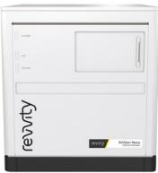
HTRF® readout can be achieved by EnVision Nexus after the installation of the HTRF® dedicated optical block which includes the optimized excitation and emission filters, the dichroic mirror and the beam splitter. The measurement conditions should then be set up in the instrument software according to the following indications:
