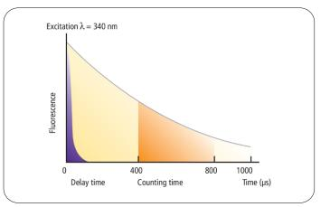
Figure 1: DELFIA time-resolved fluorescence immuno-assays dramatically improve signal detection (orange) relative to background (purple).
