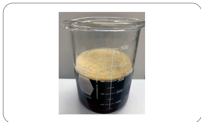
Figure 9: Pre-Processing photo of Cola sample. Note the presence of CO 2 - generated effervescence in the form of foamy-bubbles.
