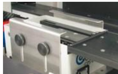
Figure 2: Integrating a Cedrex® plate holder provides a fully-automated solution for septum piercing. Compatible with either the JANUS G3 or Sciclone G3 NGS(x) Automated Workstations.
