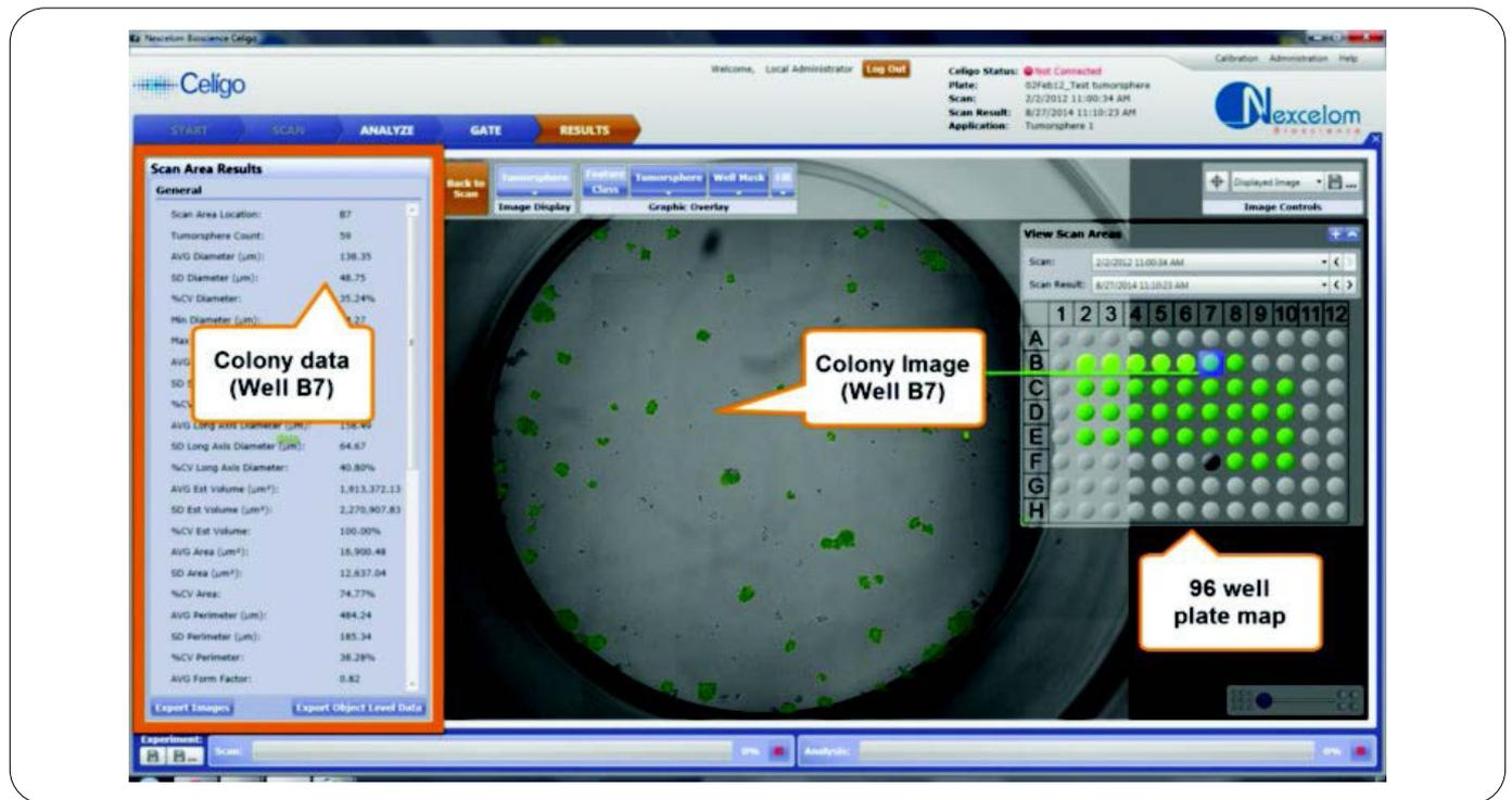
These assays utilize Celigo's brightfield imaging mode and multiple quantification methods to obtain number and size of tumorspheres cultured in 96, 48, 24, 12, and 6-well microplates, as well as 60mm dish.
