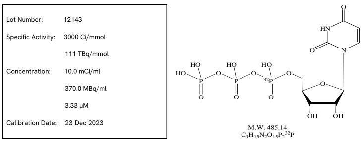
PACKAGING: 10.0mCi/ml (370.0 MBq/ml) on the Calibration Date. 50mM Tricine pH 7.6 solution and shipped in a lead container on dry ice.
