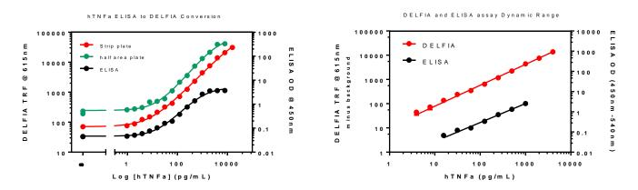
The dynamic ranges were generated using a 96-well strip plate. ELISA assay and DELFIA assay were run side by side in the separate plates. The DELFIA plate was read by an EnVision-2105 multimode plate reader with TRF flash lamp option. The ELISA plate was read on a plate reader equipped with absorbance option and the optical densities (OD) were read at 450 nm and 540 nm, respectively. ELISA kit recommended to use two wavelength readings for background correction.
