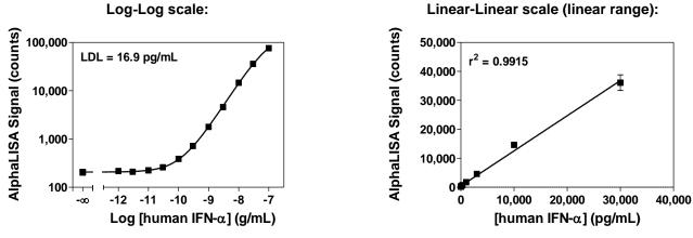
The data was generated using a white Optiplate-384 microplate and an EnVision-Alpha Reader 2102.
