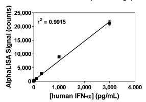
The data was generated using a white Optiplate-384 microplate and an EnVision-Alpha Reader 2102.
