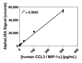
The data was generated using a white Optiplate-384 microplate and an EnVision-Alpha Reader 2102. **Manual 2 - Typical results in FBS**
