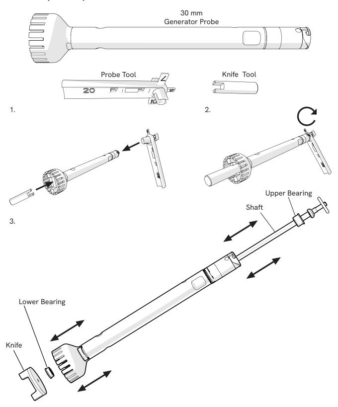
Bearing wear will be determined by factors such as frequency of use, cycle time and processing speed. Long cycle times at high speeds may accelerate bearing wear and require more frequent bearing replacement.
