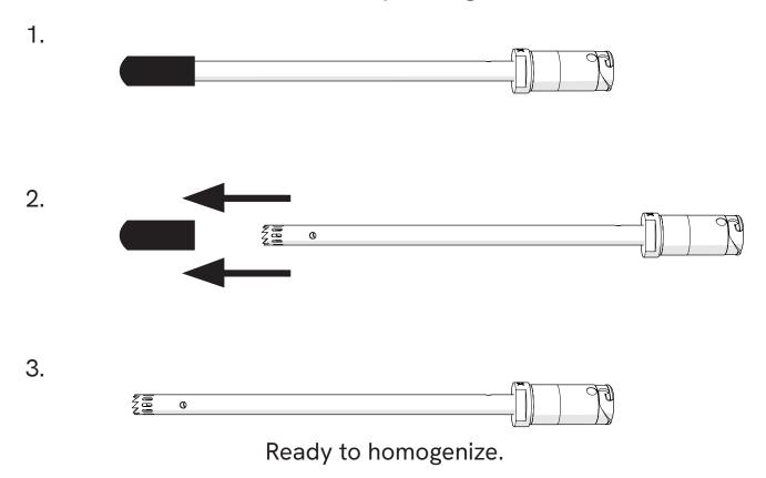
Save the blue cap to protect the probe when it is not in use.
