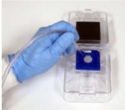
Figure 1. Using a vacuum to aspirate the chip wells is more effective than using a pipette
