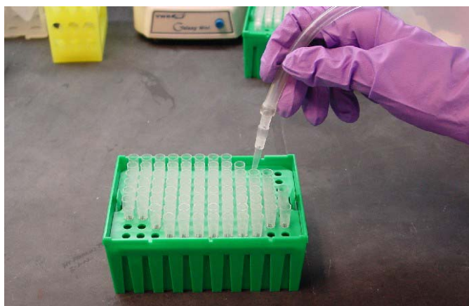
Figure 22. Replacing the disposable pipette tip
