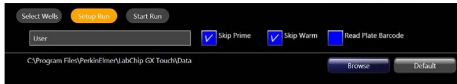
Figure 11. Setup Run tab when priming and warming takes place before the run
