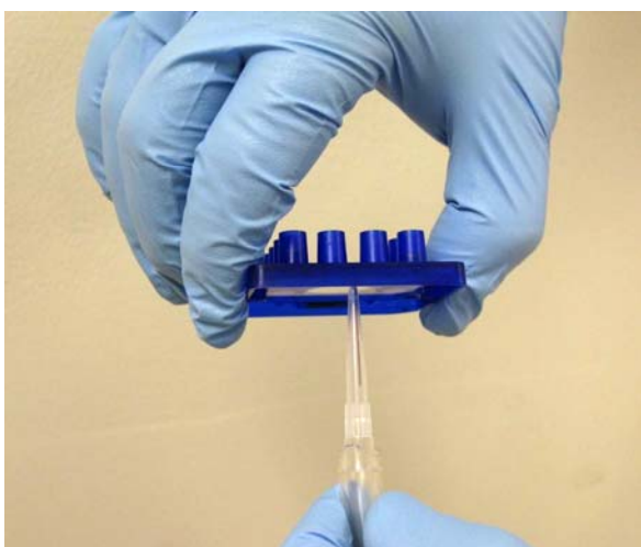
Figure 23. Removing an air bubble or clog by suctioning the sipper with a vacuum line
