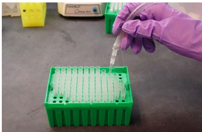
Figure 21. Replacing the disposable pipette tip.
