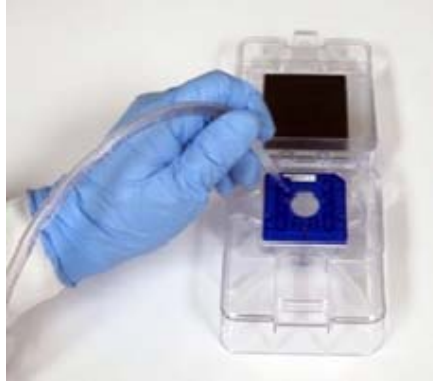
Figure 2. Using a vacuum to aspirate the chip wells is more effective than using a pipette.
