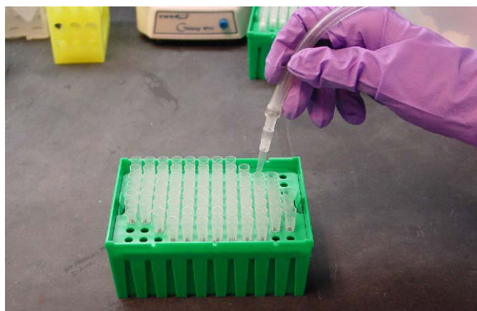
Figure 20. Replacing the disposable pipette tip.
