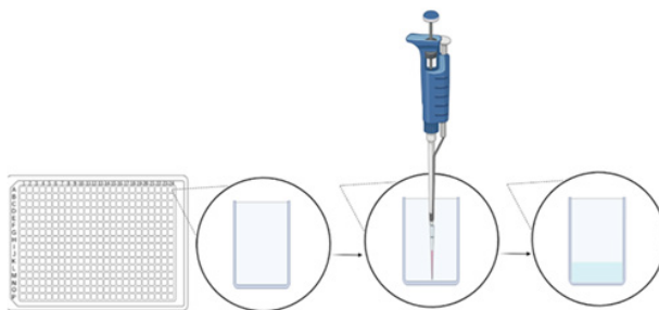
Figure 11. Pipetting directly at bottom of wells
