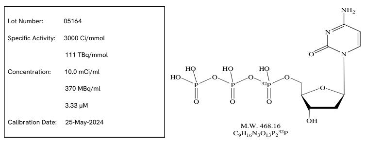
PACKAGING: 10.0mCi/ml (370 MBq/ml) on the Calibration Date in a 50mM Tricine pH 7.6 solution containing a stabilizer.\* A green dye is added as a visual aid for pipeting. The product is shipped ambient in a plastic container. The lead-free container is non-toxic and environmentally friendly.
