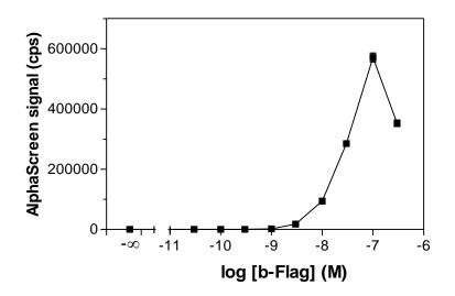
**Figure 1:** Biotinylated-probe titration assay 384-well biotinylated-FLAG titration curve (25 µL final volume; Reader: Envision). Note: Alpha signal will vary depending on instrument detection protocol, incubation temperature and incubation time.
