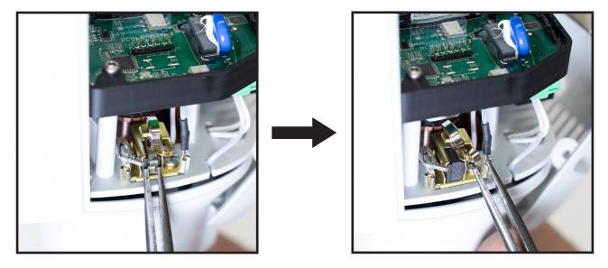
6. Using needle nose pliers, carefully place the coil spring onto the coil spring tab of the brush holder.
