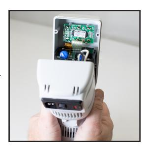
1. Remove the four Phillips screws from the back of the unit.
