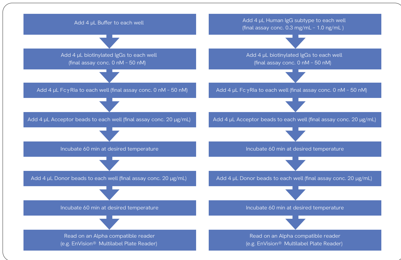
Figure 4: Assay diagram showing the steps used in the titration binding assay (left side) and competition assay (right side).
